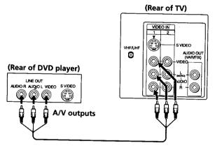
For optimum picture quality, use S VIDEO instead of the yellow A/V cable. S VIDEO does not provide sound, your audio connectors must still be connected.
