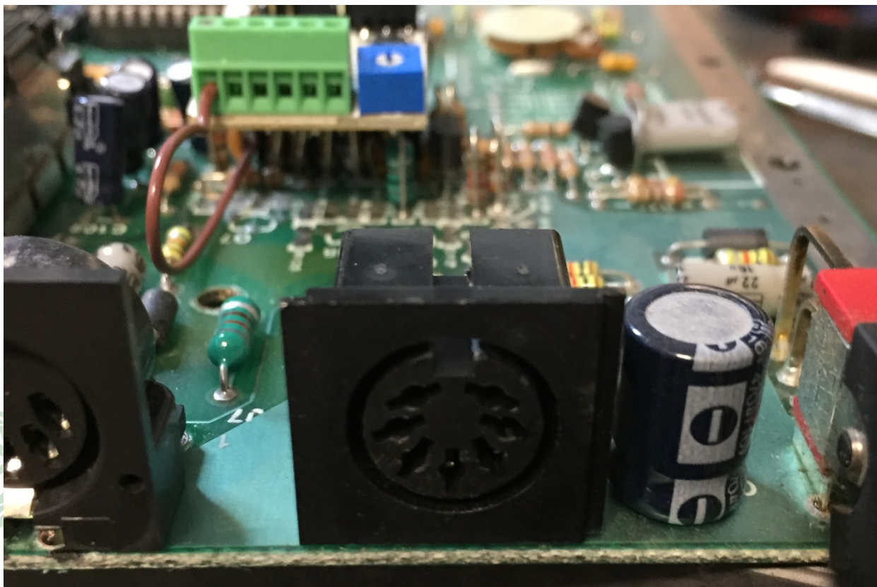
Figure 7: DIN5 installed (top)
