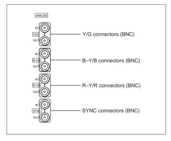
RGB signals, component signals (Y, R–Y, and B–Y), or composite sync signals can be fed in the IN connectors. The type of signal applied to each connector is set with the INPUT CONFIGURATION menu. The OUT connectors are used for loop-through output of the input signal. When not using loop-through, connect a 75-ohm terminator (not supplied) to the OUT connectors.
