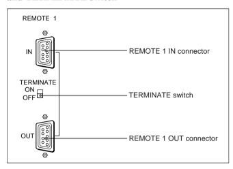
These are RS-485 serial interface connectors, used for connecting two or more BVM-series monitors. The IN and OUT connectors form a loop-through connection. Set the TERMINATE switch to OFF. Connect two monitors using a straight cable with D-sub 9-pin plugs such as an RCC-5G (not supplied) as shown in the figure.
