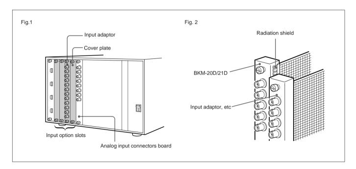
When installing adaptors, moving the analog input connectors board, or fitting a cover plate over an unused slot, always **fit the BKM-20D/21D as the last step of the operation**. If a BKM-20D/21D is already installed, remove it temporarily while carrying out the other operations, then reinstall it last.
