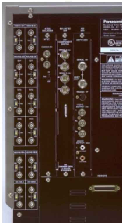
The AT-H1915 DA with optional boards (NTSC decoder, 601 component digital I/F and HD component digital I/F). An NTSC composite digital IF board is also available.
