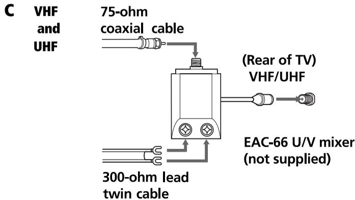
This allows you to connect your TV to both a cable system and a dipole antenna, in order to view both cable and local channels.
