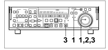
**1** Press the SHUTTLE button or search dial so that the SHUTTLE button is lit.
