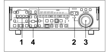
**1** Press the appropriate INSERT button (VIDEO, CH-1 to CH-4, or TIME CODE).
