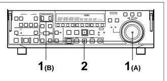
**1** (A) Hold down the PLAY button, and turn the search dial in the desired direction to adjust the playback speed.
