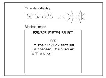
**4** Holding down the JOG button, turn the search dial to change the setting from "525" to "625".
