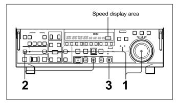
1 Hold down the DMC EDIT/FEED button, and turn the search dial to set the playback speed.
