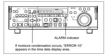
If this happens, the drum and capstan motors stop and the cassette is automatically ejected. Then, the durm starts to rotate again to dry its surface. In this state, the unit is not operable. When the moisture has evaporated, the error message disappears and the ALARM indicator goes off.
