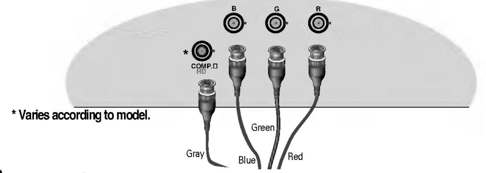
3. In case of using a separate horizontal and vertical sync signal: Connect each R, G and B video signals and the horizontal and vertical sync signal to BNC receptacles on rear panel.
