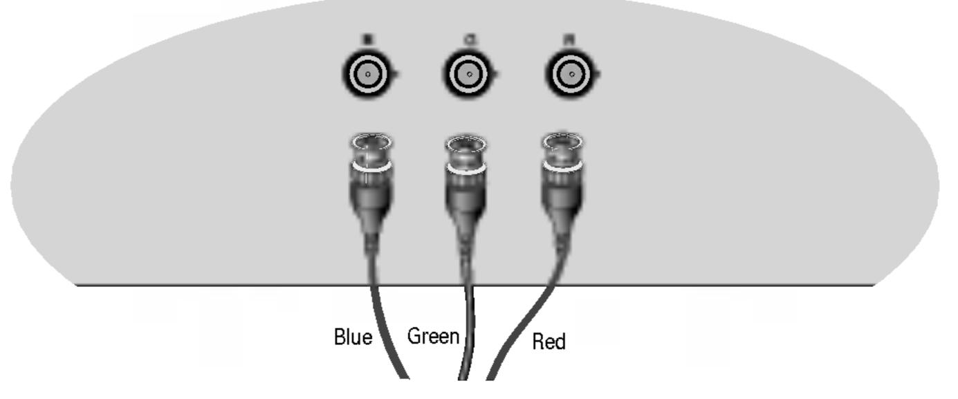
2. In case of using an external composite sync signal: Connect each R, G and B video signals and composite sync signal to the BNC receptacles on the rear panel.
