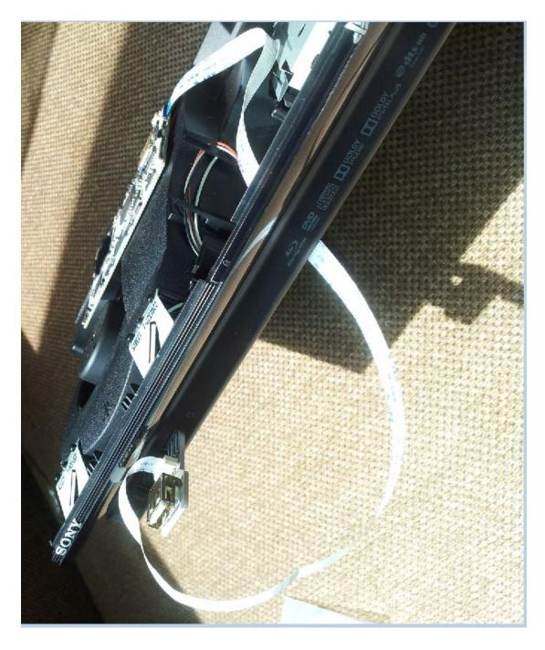
The E3 ODE PRO should be positioned inside the console as shown (CECH25XX/3XXX):
