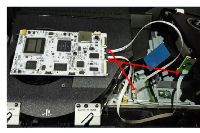
On other console which hasn't 6PIN connector like 25xx, user needn't connect those 6PIN cable.
