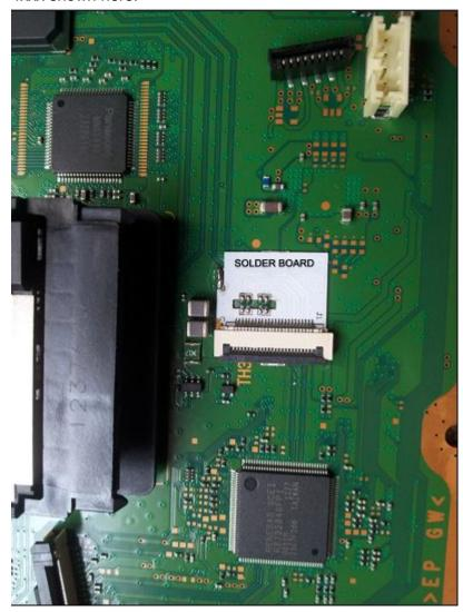
Then insert the 24 pin FFC LVDS cable (Marked as F the table above) between solder board on the ODE and 24 pin FFC LVDS connector on the solder board which you soldered to the console motherboard.
