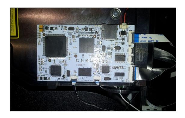
The E3 ODE PRO should be positioned inside the console as shown (CECH4XXX):
