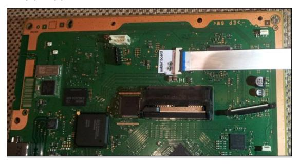
Route the FFC cable out of the shielding as shown: 25xx/3xxx shown here:
