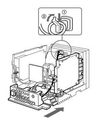
13 Fasten the cables to the G board.
