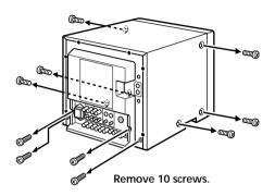
2 Remove the G board and attach it again as in the illustration.
