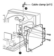
Wind the cable connected to the D board to the supplied ferrite core (large) by two turns and fasten the cable with the cable clamp.
