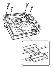
4 Connect the CN1 terminal on the BA board to the CN3 teminal on the BV board, and connect the CN2 terminal on the BA board to the CN4 terminal on the BV board, using the connecting cables supplied with BKM-102.
