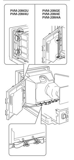
11 Install the G board (removed in step 2) as it was.
