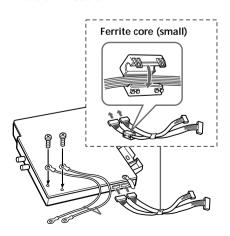
7 Connect the SDI module and the supplied BB board to the monitor board.
