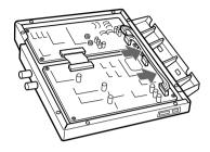
**6** Attach the cover of the SDI module using the 8 screws removed in step **1**.
