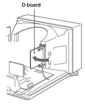
Install the supplied cable clamp (Ø11) and wind the cable connected to the D board to the supplied ferrite core (large) by two turns and fasten the cable with the cable clamp.
