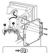
Push the SDI module forwards (to the display side), and fasten it with screws.
