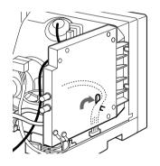
15 Make two holes for connectors of the SDI module on the rear cover of the SDI module on the rear cover of the monitor, and stick the connector label beside the holes.
