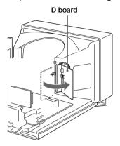
2 Connect the 12-pin connector of the SDI module to the CN8 terminal (white) of the BB board, and connect the 6-pin connector of the SDI module to the CN5104 terminal (black) on the D board.
