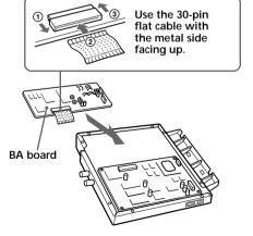
Insert the 30-pin flat cable connector into the CN5 terminal on the BV board, and secure the BA board using the supplied 4 screws with BKM-102.
