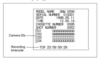
The details in the shot data depend on the shooting conditions. If because of the devices used there is no shot data on a part of the tape, it appears as blank.
