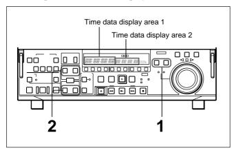
1 Press the RECORDER button or PLAYER button to select the VTR on which you wish to check the edit point.
