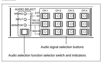
When the MIXING indicator is lit: You can use the EXT and REC CH rows of the audio signal selection buttons to switch the audio signals to be recorded or carry out mixing.
