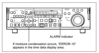
If this happens, the drum and capstan motors stop and the cassette is automatically ejected. Then, the durm starts to rotate again to dry its surface. In this state, the unit is not operable. When the moisture has evaporated, the error message disappears and the ALARM indicator goes off.
