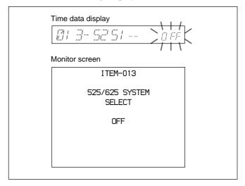
**2** Holding down the JOG button, turn the search dial to change the setting from "OFF" to "ON".
