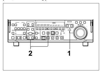
Press the RECORDER button or PLAYER button to select the VTR on which you wish to operate.
