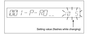
**2** When the desired setting value is displayed, press the SET button.
