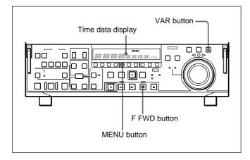
Press the MENU button, turning it on. The F FWD button and VAR button light, and the setting of the currently selected menu item appears in the time data display area 1 and 2.
