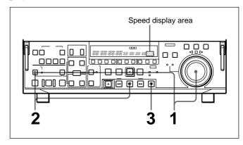
1 Hold down the DMC EDIT/FEED button, and turn the search dial to set the playback speed.
