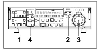
Press the appropriate INSERT button (VIDEO, CH-1 to CH-4, or TIME CODE).
