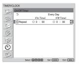
4 When you want to apply the setting to every day of week, change ○ to ○ and press ENTER. If you press ENTER with the radio button set to ○, the setting will be only applied once.
