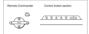
Operation of the unit is explained in these operating instructions for the case of operation using the Remote Commander. The  $\uparrow/\downarrow$  and ENTER buttons on the Remote Commander have the same functions as the  $\uparrow/\downarrow$  and ENTER buttons on the display.
