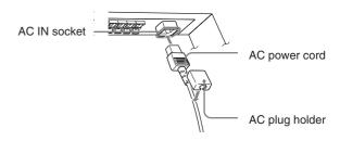
**2** Slide the AC plug holder over the cord until it connects to the AC IN socket cover.
