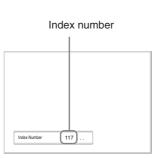
2 Input the index number of the display you want to operate using the 0-9 buttons on the Remote Commander.
