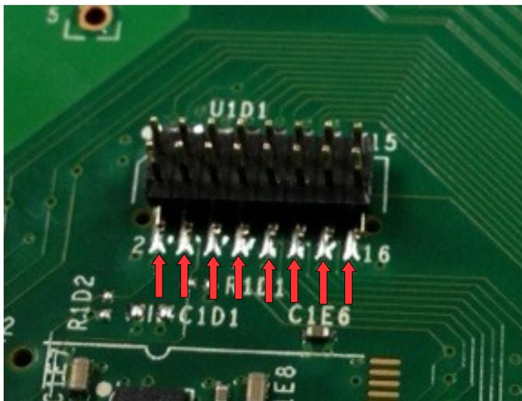
–Attach a Single wire from Oscillator to PIN 15 of header
