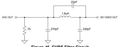
Figure 46. CVBS Filter Circuit
