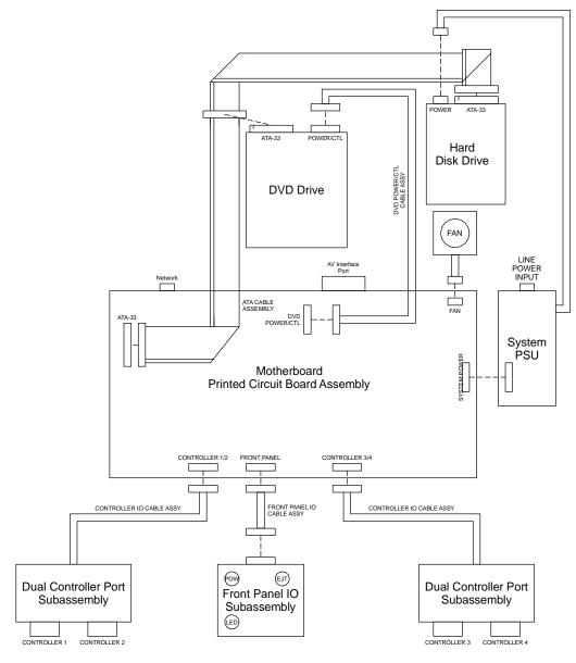
Figure 82. Xbox Top-Level Assembly Block Diagram
