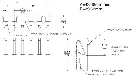
Figure 96. System Power Output Connector Header
