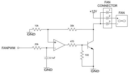
Figure 20. Fan Speed Control Circuit
