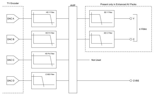
Figure 45. Video Filter Arrangement, SDTV Mode
