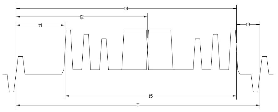
This appendix contains a summary of the horizontal timing specifications for the Y, Pb, and Pr video output waveforms. Refer to the timing diagram above for the measurement reference points for HDTV modes. This line drawing is a composite of the various landmarks generated from the timing test signal pattern described in Appendix I.
