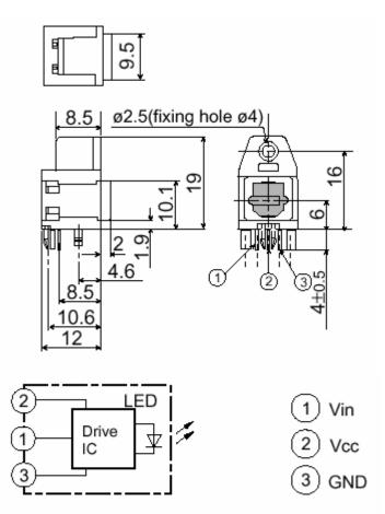
Figure 42. SP-DIF Optical Transmitter Module
