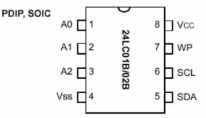
Figure 27. Configuration EEPROM pin out
