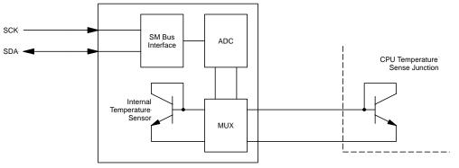
Figure 19. Temperature Monitoring Circuit
