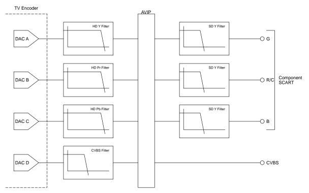
Figure 49. Video Filter Arrangement, Component SCART Mode
