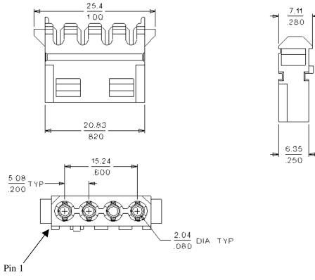
Figure 97. Disk Drive Power Connector
