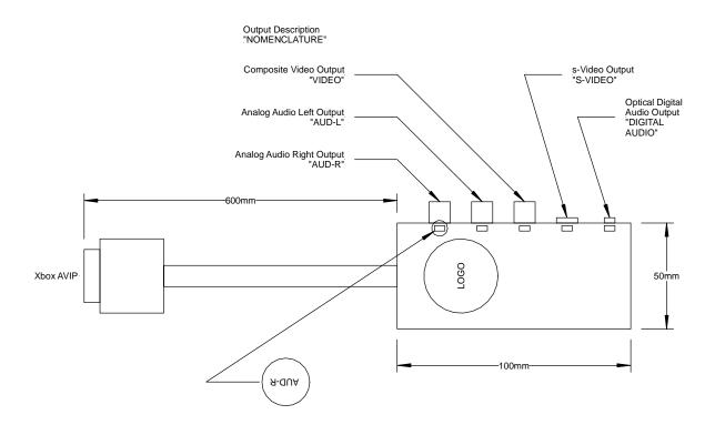
Figure 73. Enhanced NTSC A/V Pack Mechanical Layout
