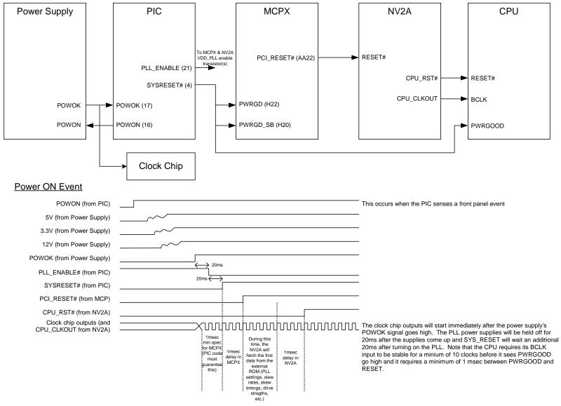
Figure 102. System RESET Control Flow
