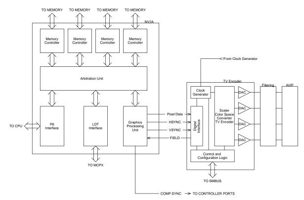
Figure 6. Graphics Subsystem Block Diagram
