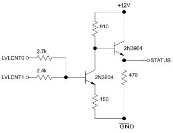
Figure 56. SCART Status Output Circuit
