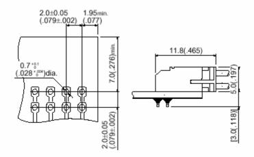
Figure 34. DVD Power and Control Interface Connector
