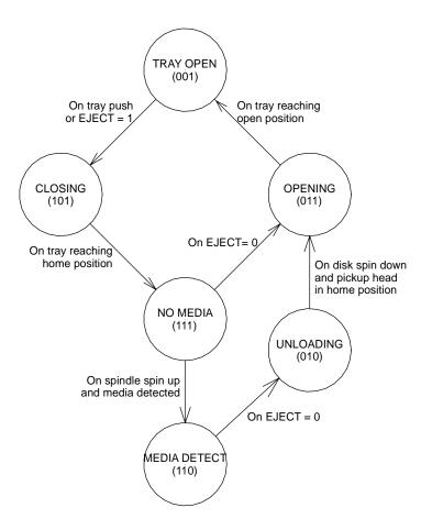
Figure 35. DVD Mechanism State Diagram
