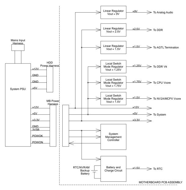
Figure 67. Power Supply Block Diagram
