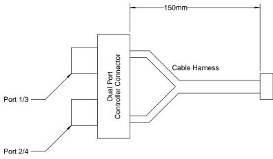
Figure 95. Dual Controller Port Subassembly
