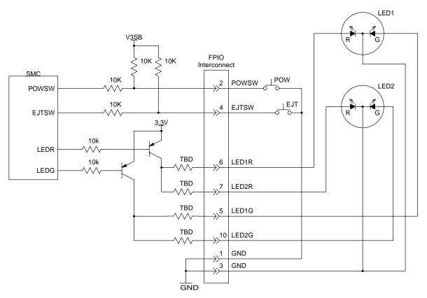
Figure 22. Front Panel IO Schematic
