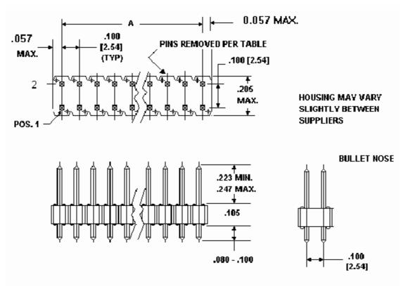
Figure 65. LPC Interface Header (Dimension A=0.70 inches)
