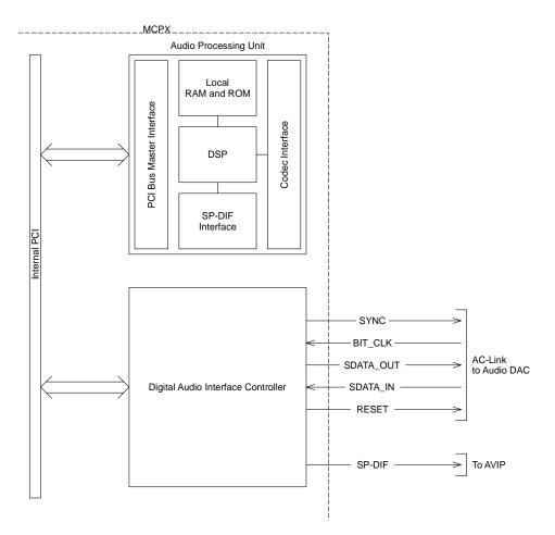
Figure 11. Audio Subsystem Block Diagram
