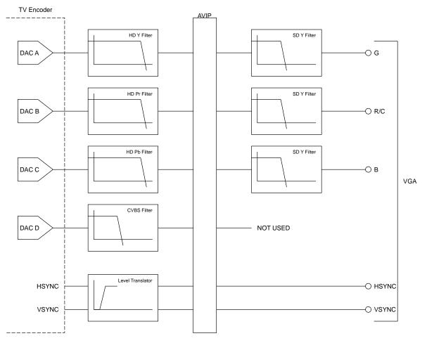
Figure 53. Video Filter Arrangement, Component SCART Mode
