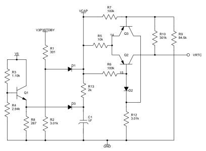
Figure 70. RTC Holdup Circuit
