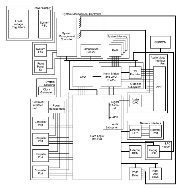
Figure 2. Xbox System Block Diagram
