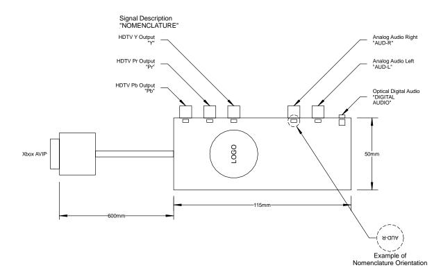
Figure 81. HDTV AV Pack Mechanical Layout
