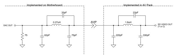
Figure 47. SD (Y and C) Filter Circuit
