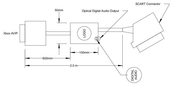
Figure 74. Enhanced SCART AV Pack Mechanical Layout
