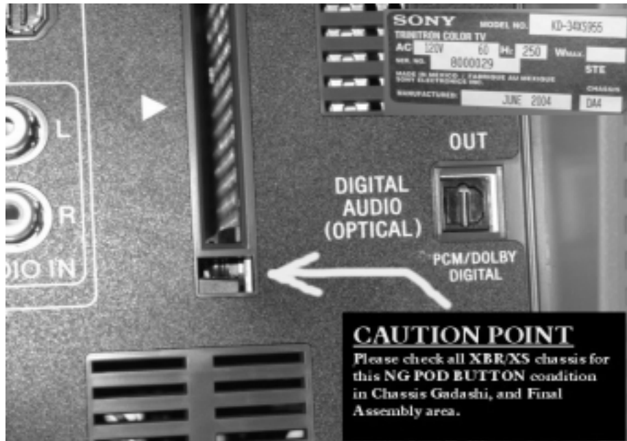
This was a defect from Pre-Pro set. Important to check alignment of POD Eject Button. VERY important if QBOX is replaced in the field.
