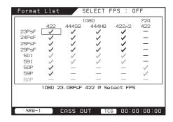
A bar appears for formats that cannot be used. A yellow or green check mark appears for formats that can be used. The check mark is green for formats that can be used when the SELECT FPS function is enabled.
