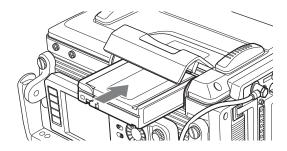
**4** Press the cover of the cassette insertion slot to close it. The tape is wound on the drum.
