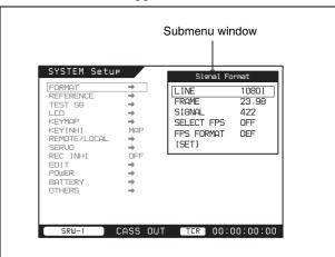
**3** Rotate the SELECT/ENTER dial to select LINE in the submenu window.
