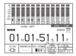
The S in S23PsF indicates that SR Motion is enabled. (SELECT FPS is set to "ON" for Slow Shutter.) The 23PsF indicates that FPS FORMAT is set to 23.98PsF. (23PsF) indicates that the target frame frequency is 23.98PsF.
