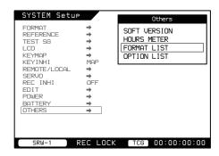
**3** Rotate the SELECT/ENTER dial and select FORMAT LIST in the submenu window.
