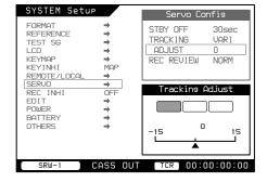
While viewing the channel condition display, rotate the ADJUST knob or SELECT/ENTER dial to adjust so that the channel condition display lights in green.
