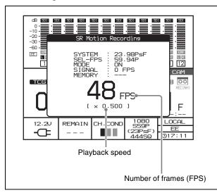
To confirm the new setting, press the SELECT/ ENTER dial or leave it unrotated for three seconds. The display returns to the original screen.
