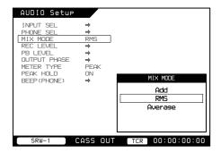
Rotate the SELECT/ENTER dial to select the mixing method.
