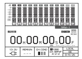
Recording at the specified intervals of specified time begins, and the specified number of frames are accumulated in the memory of the HKSR-102. Recording to tape starts when the amount of data reaches the specified amount. The tally indicator of this unit lights during storage to memory and during recording to tape
