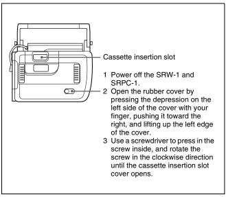
There is no need to return the screw to its original position after you remove the cassette. Normal operation resumes again the next time you power the system on.
