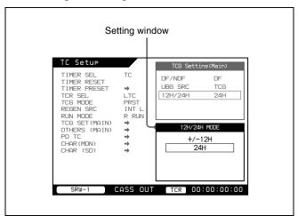
**4** Rotate or press the SELECT/ENTER dial to select the desired setting.
