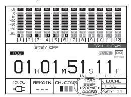
The S in S59P indicates that SR Motion is enabled. (SELECT FPS is set to "VTR", and the Interval Frame function is used.) The 59P indicates that FPS FORMAT is set to 59.94P. (23PsF) indicates that the target frame frequency is 23.98PsF.
