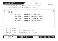
**3** Rotate the SELECT/ENTER dial to select the bank into which to load the LUT file, and then press the dial.
