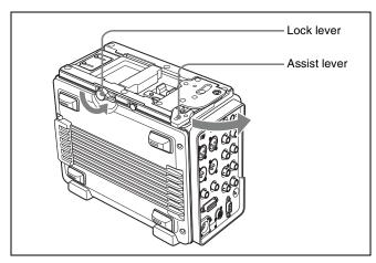
4 Grasp the top handle of the SRW-1, align the I mark on the SRW-1 with the ▲ mark on the SRPC-1 (see "To release" in the following figure), and then place the SRW-1 on the top of the SRPC-1.
