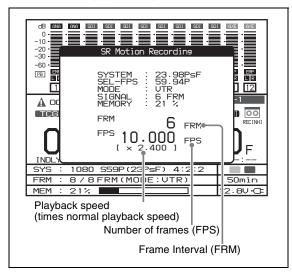
When you press the SELECT/ENTER dial with the FUNC button held down and do not perform any operation for three seconds, the screen returns to the previous state. When you press the SELECT/ENTER dial with the FUNC button held down and press the SELECT/ENTER dial again with the FUNC button held down, the following screen appears. This screen remains on the display even if you do not perform any operation for three seconds or more.
