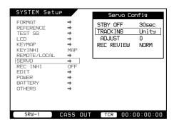
When the tracking has been automatically optimized, the tracking control is not released even if the cassette is ejected or the system is powered off.
