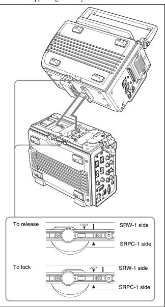
8 Rotate the assist lever back to its original (lock) position to align the LOCK ▼ mark on the SRW-1 with the ▲ mark on the SRPC-1. (See "To lock" in the previous figure.)
