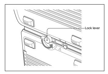
4 While pulling out the release knob on the side panel of the SRPC-1, rotate the assist lever in the direction of arrow and then slide the SRW-1.
