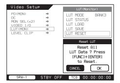
**2** Rotate the SELECT/ENTER dial to select OK, and then press the dial with the FUNC button held down.
