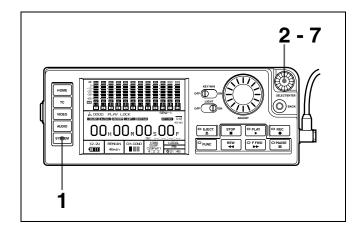
**1** Press the menu selection button "SYSTEM" on the control panel.
