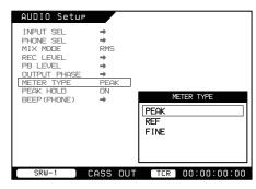
Rotate the SELECT/ENTER dial to select the scale to display.
