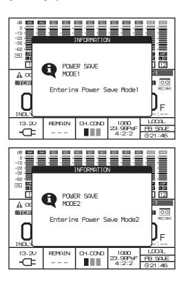
In addition, "xx SAVE" appears on the second line of the status indication in the display, and the "SRW-1" indication under the audio level meters change as follows.
