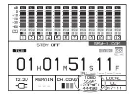
The S in S59P indicates that SR Motion is enabled (SELECT FPS is set to "ON"). The 59P indicates that FPS FORMAT is set to 59.94P. (23PsF) indicates that the target frame frequency setting is 23.98PsF.
