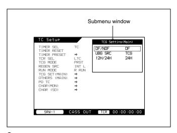
**3** Rotate the SELECT/ENTER dial to select the desired setting in the submenu window.
