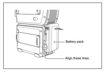
3 Slide the battery pack down until its LOCK arrow points at the matching line on the SRPC-1.
