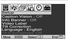
Select closed captioning options, display the name of the currect program and its remaining time, label video inputs, adjust tilt correction (available only for KV-25FS120), select menu languages, or run a demo of the menus.
