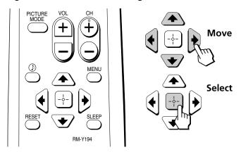
To navigate on the on-screen menus, use the "arrow" buttons ( $\spadesuit$ ,  $\blacktriangledown$ ,  $\spadesuit$ ) to move the cursor. Pressing these arrows will cause the cursor to move in the corresponding direction. Pressing center button  $\bigoplus$  will allow you to select an option.
