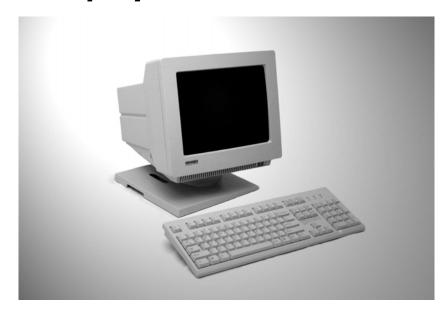
The ADDS 4000/260 has advanced data access, data manipulation and display features, including cut and paste and dual host/dual session capabilities. The terminal features selectable refresh rates up to 100Hz for clear, flicker free viewing and an ISO 9241.3 compliant mode to reduce operator eye strain. Bezel to bezel over scan is also available up to 82 Hz.
