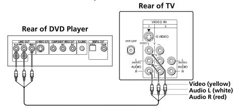
For better picture quality, use S VIDEO instead of the yellow Audio/ Video cable. S VIDEO does not provide sound; the audio cables must still be connected.
