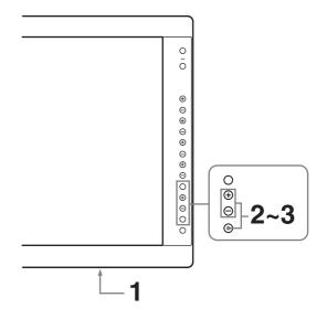
**1** Turn on the unit with the  $\odot$  /  $\circlearrowleft$  (power) switch on the bottom panel.
