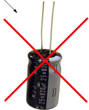
CAPACITOR IN SERVICE MANUAL (1-111-066-11) 820 µF/25V, 105°C (12.8 mm DIAMETER x 20)
