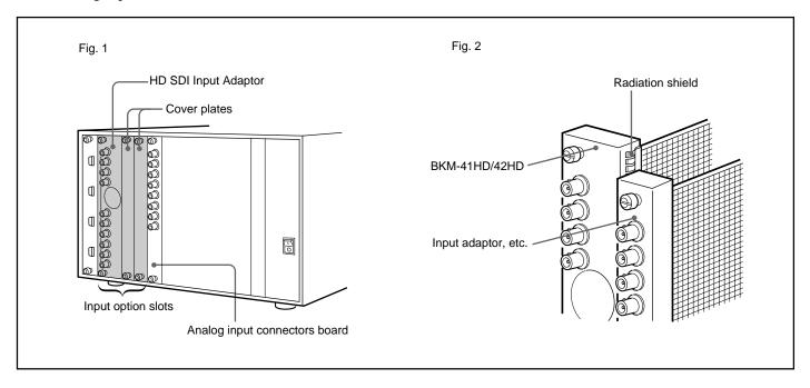
When installing adaptors, moving the analog input connectors board, or fitting a cover plate over an unused slot, always **fit the BKM41HD/42HD at the last step of the operation.** If a BKM-41HD/42HD is already installed, remove it temporarily while carrying out the other operations, then reinstall it last.
