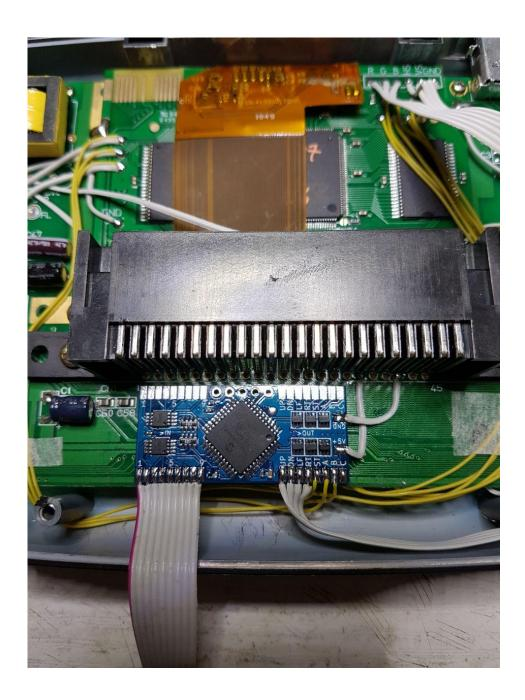
Referring to the picture above, on the bottom right you can see a row of solder pads labelled UP,DN,LF,RT,ST,A,B,C
