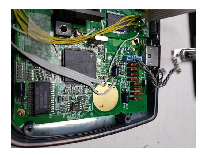
If you have the McWill LCD replacement screen installed, then you can common the button inputs by attaching directly to the screen connections as shown below.
