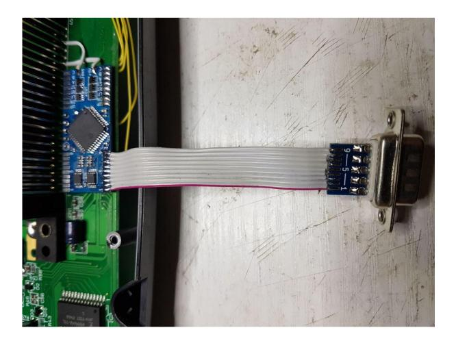
Now, solder the other end of the IDC cable to the processor board, observing polarity as indicated on both PCB's and the red IDC wire indication.
