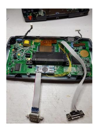
The Scope of this Guide is to aid the Installation of the Pxlmod SEGA Game Gear Controller kit which can be purchased from VideoGamePerfection.Com. It allows the connection of a regular SEGA MegaDrive Joypad to control the Game Gear.
