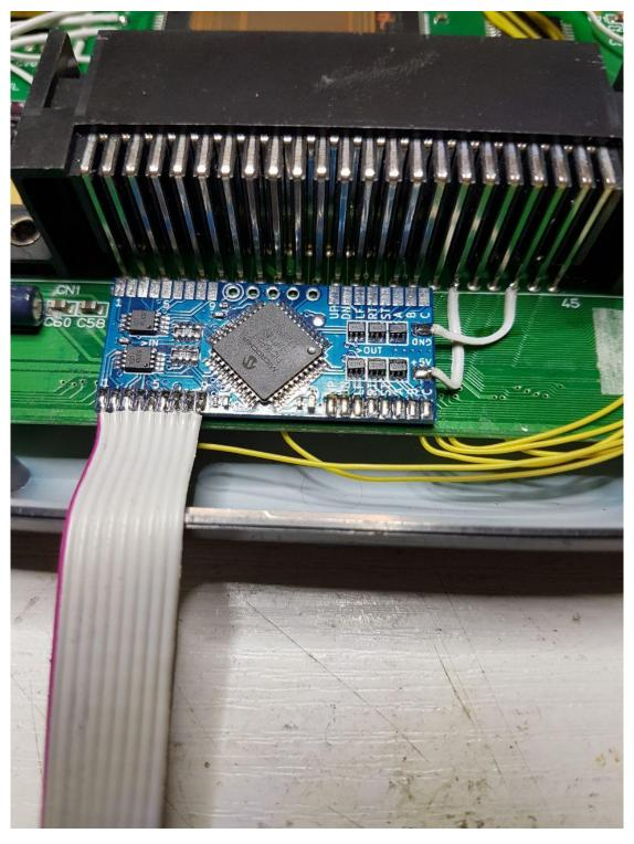
Ensure you leave a gap between the processor PCB edge and the Game Gear cartridge pins.
