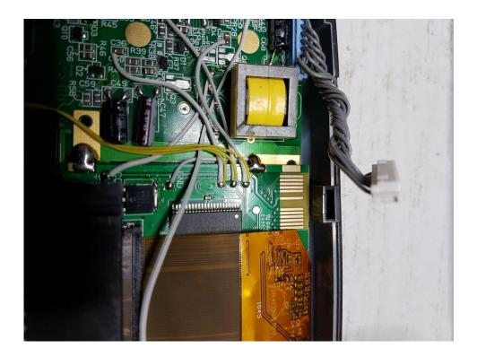
Otherwise just solder the button wires directly as outlined in the Table to the left hand side of the Game Gear PCB.
