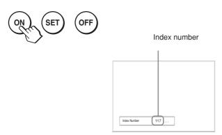
**2** Input the index number of the display you want to operate using the 0 – 9 buttons on the Remote Commander.
