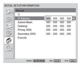
3 Set the three digit value (0 to 255) for the first box with ↑/↓ on the display unit or numeric keys on the remote commander and press ENTER or →.
