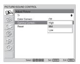
2 Select the Gamma Correct. mode with ↑/↓. High: Sets the Gamma Correct. to high. Mid: Sets the Gamma Correct. to medium.
