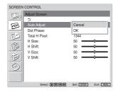
(2) Select "OK" with **↑**/**↓** and press ENTER. All the items of "Adjust screen" menu are adjusted automatically.
