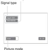
You can switch the input signal using the OPTION button on the display unit.
