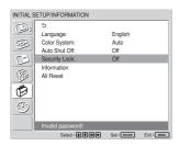
**4** After completing the process described above, turn off the display unit and unplug the power cord to make the setting valid.
