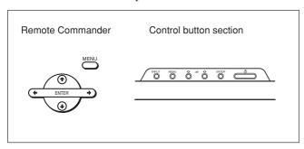
Operation of the unit is explained in these operating instructions for the case of operation using the Remote Commander. The ↑/♣ and ENTER buttons on the Remote Commander have the same functions as the ↑/♣ and ENTER buttons on the display.
