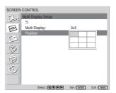
7 Select the position of this particular display unit in the arrangement of the video wall with 1/4/4-/
