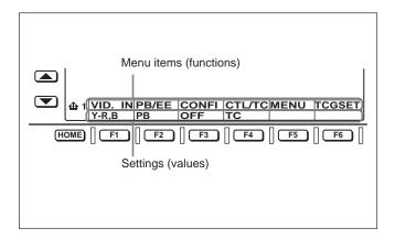
In the figure above, Y-R,B (analog component signals) is selected as the setting for VID.IN, the menu item for button F1. This manual refers to this as "F1 (VID.IN) in function menu HOME page is set to Y-R,B."
