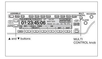
When the menu item number displayed in the menu display is flashing, you can change the menu item by turning the MULTI CONTROL knob.
