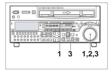
1 Press the SHUTTLE button or search dial so that the SHUTTLE button is lit.
