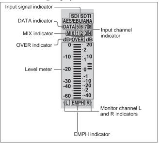
**Input signal indicator:** Indicates the currently selected input signal ('SDI', 'SDTI', 'AES/EBU', 'ANA' for analog) for the corresponding audio input channel.
