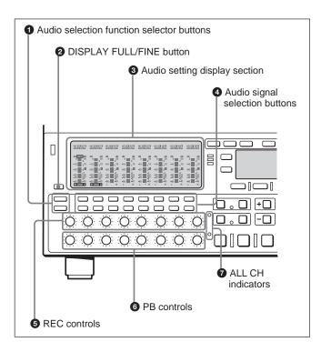
In the audio control section, you can select and display input and output signals for audio channels 1 to 8. Depending on the number of audio recording channels, the indication of the format during tape playback changes to an indication of the channels that can be set.
