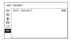
You can lock the setting so that they cannot be changed by an unauthorized user.
