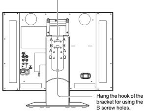
**5** Secure the arm with four screws.
