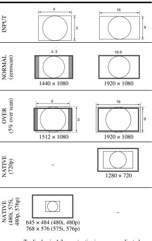
To display in 4:3 aspect ratio, images are adjusted horizontally with scale handling.
