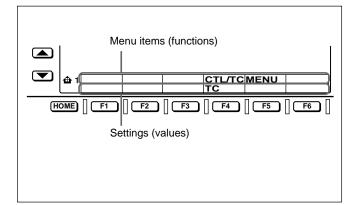
In the figure above, TC (time code) is selected as the setting for CTL/TC (time data selection), the menu item for button F4. This manual refers to this as "F4 (CTL/TC) in function menu HOME page is set to TC."
