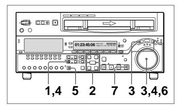
Press the DMC EDIT button, turning it on.
