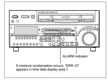
If this happens, the drum and capstan motors stop and the cassette is automatically ejected. Then, the durm starts to rotate again to dry its surface. In this state, the unit is not operable. When the moisture has evaporated, the error message disappears and the ALARM indicator goes off.
