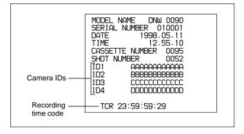
The details in the shot data depend on the shooting conditions. If because of the devices used there is no shot data on a part of the tape, it appears as blank.
